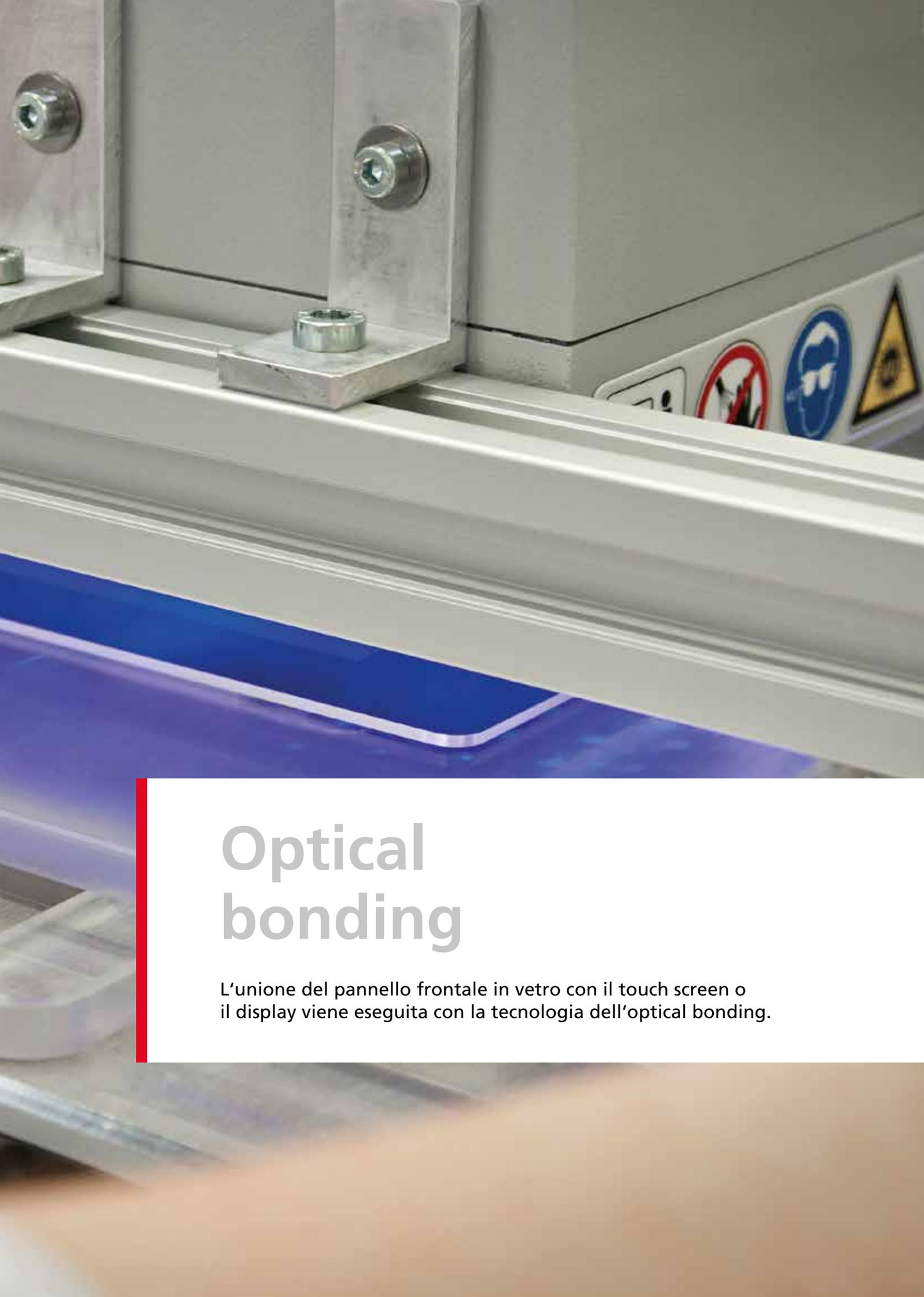
A close-up photograph of an industrial machine, likely used for optical bonding. The machine has a grey metal frame with several silver-colored metal brackets and bolts. A blue-lit glass panel is visible in the foreground. On the right side of the machine, there are several safety warning signs, including a red circle with a slash, a blue circle with a white figure, and a yellow triangle with a black exclamation mark.
