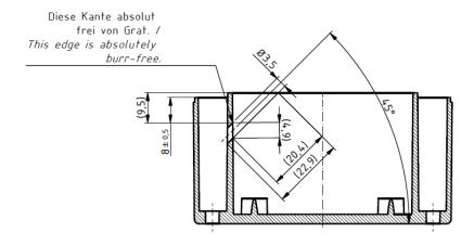
DAE-D11 is glued on from the inside, centrally to the contour. Piercing from the outside is not possible.
