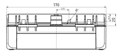
Glue the DAE-D11 from the inside centrally to the contour. Penetration from outside after the hinged catches have been activated is not possible.
