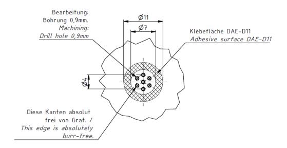
Drill the 0.9 mm hole pattern and glue-in the DAE-D11 from the inside and centrally.
