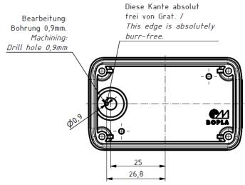
Drill the 0.9 mm hole from the inside and glue the DAE-D11 into the round contour.
