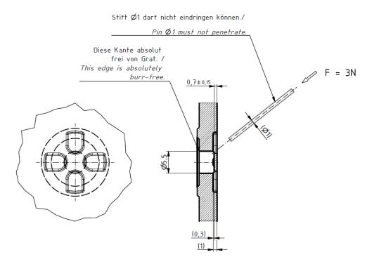
Mill the deep drill hole from the inside and glue the DAE-D11 from the inside into the round contour. Installation situation for BOCUBE Concealed by the hinged catch.
